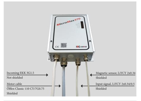
EMC glands must be used for shielded cables.
