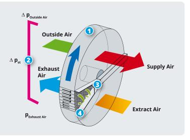
The table below lists guideline values for possible use of a purge chamber. Since the purge pressure in [Pa] plays an important role and the purge air volume must always be higher than the extract air volume transferred via rotation, use of the Klingenburg design software is recommended to determine whether a purge chamber is effective and if so, which size.
